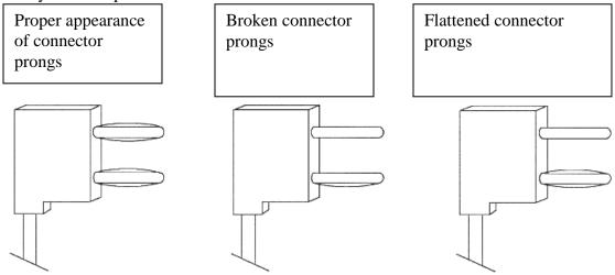
Figure A-4 Inspect Touchpad and Button Connectors
