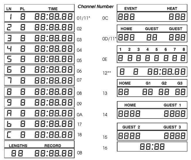
Figure 2-K Scoreboard Displays/Channel Numbers
