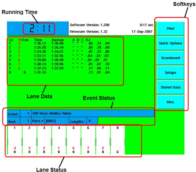
Figure 4-A Main Menu Screen with Features Labeled
