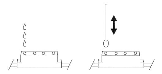
Figure A-3 Clean Cable Connectors as shown
