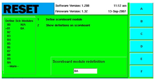
Figure 4-H Scoreboard Module Definition Window
