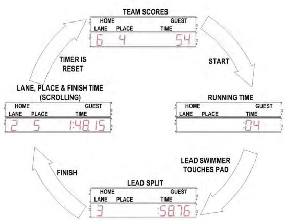
Figure 2-I Single-line Scoreboard Display Sequence
