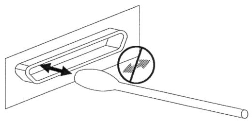
Figure A-2 Clean Data Connectors as Shown
